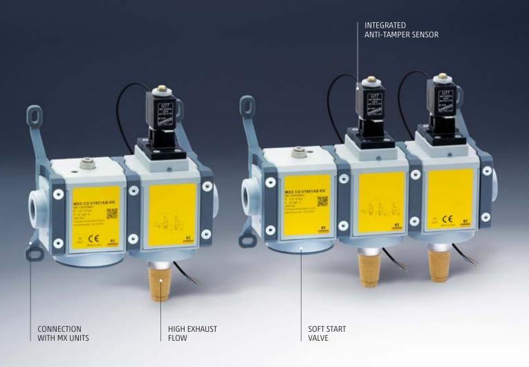
The new Series MX SAFEMAX soft start valve enables gradual pressurisation of the system, while maintaining all safety functions.
